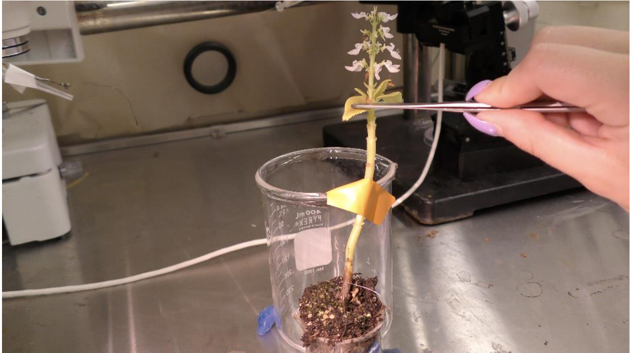
Figure 5: Bending a leaf while recording using impedance technique.
