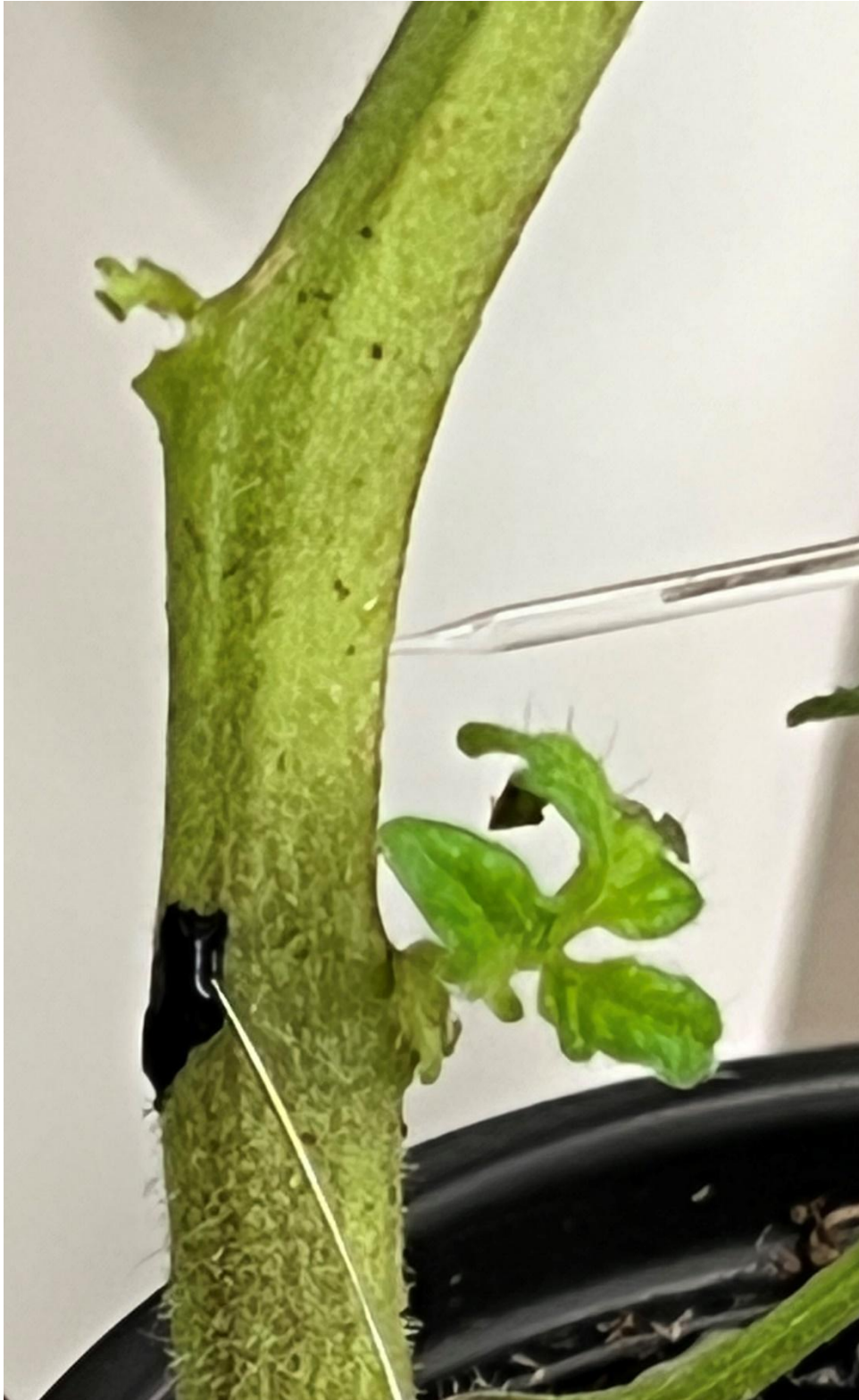
Figure 1: A representative tomato plant with a glass electrode placed within the stem and the ground wire attached to the stem with conductive black paint.
