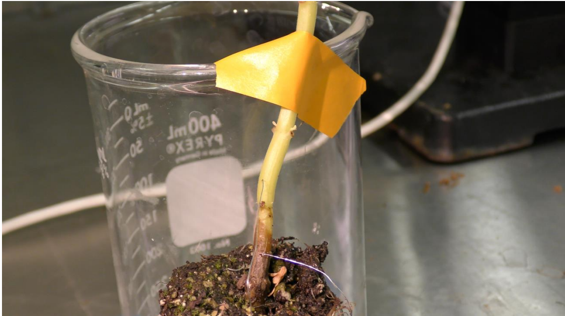
Figure 4: Impedance wires placed in (penetrated) the stem of Coleus scutellarioides .
